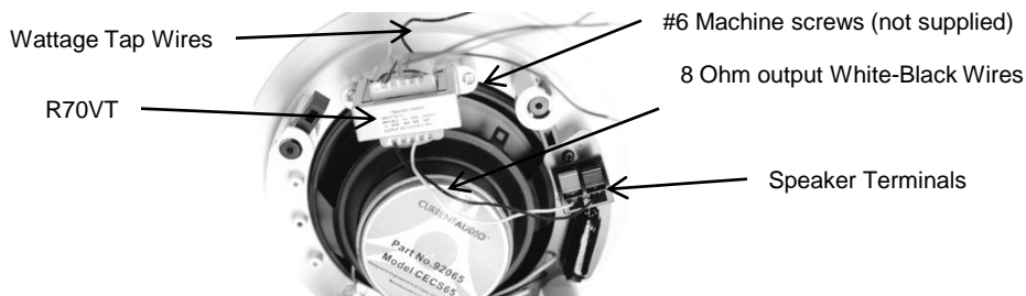
Typical Transformer Mount, CECS65 Shown
