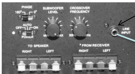
LINE INPUT (LFE) Connection
